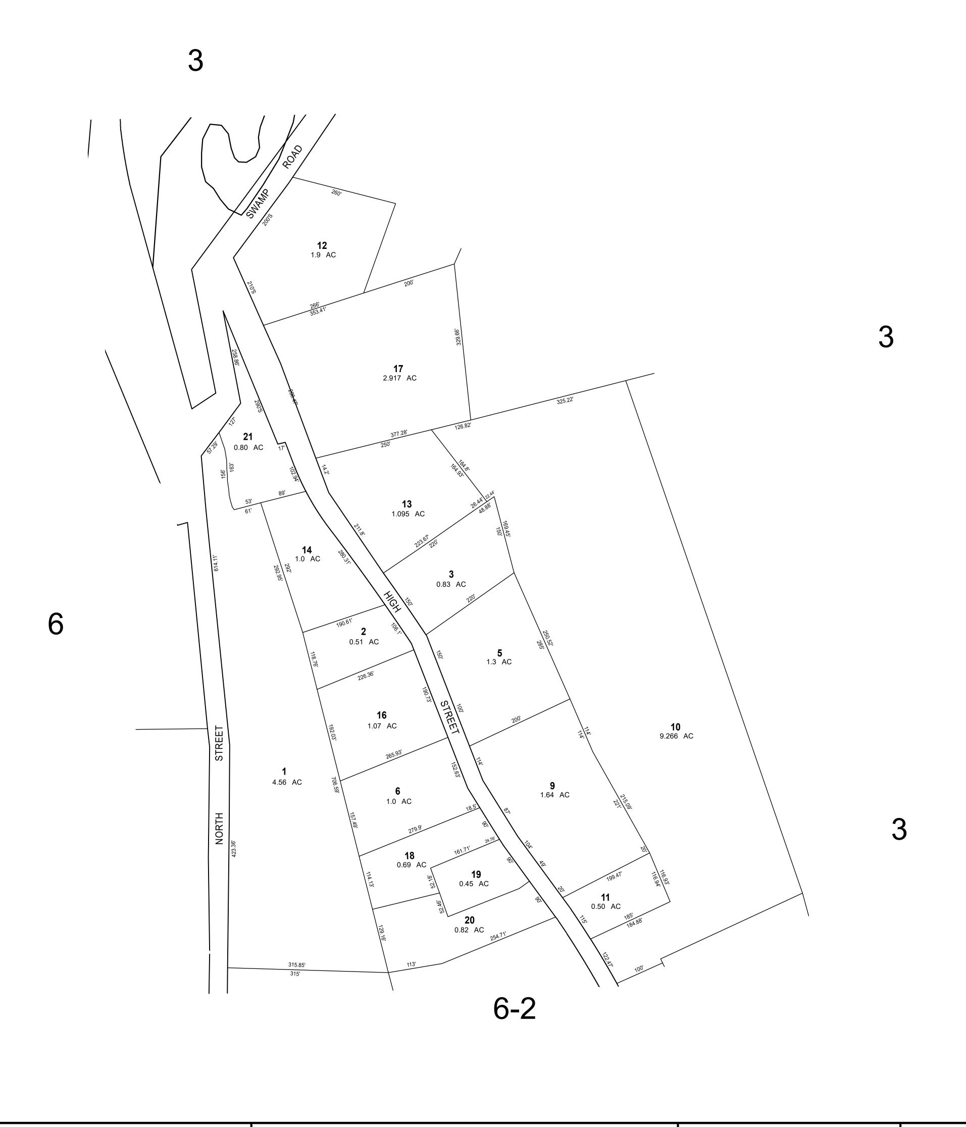
THE HORIZONTAL DATUM IS THE MASSACHUSETTS STATE PLANE COORDINATE SYSTEM, NAD 83.
