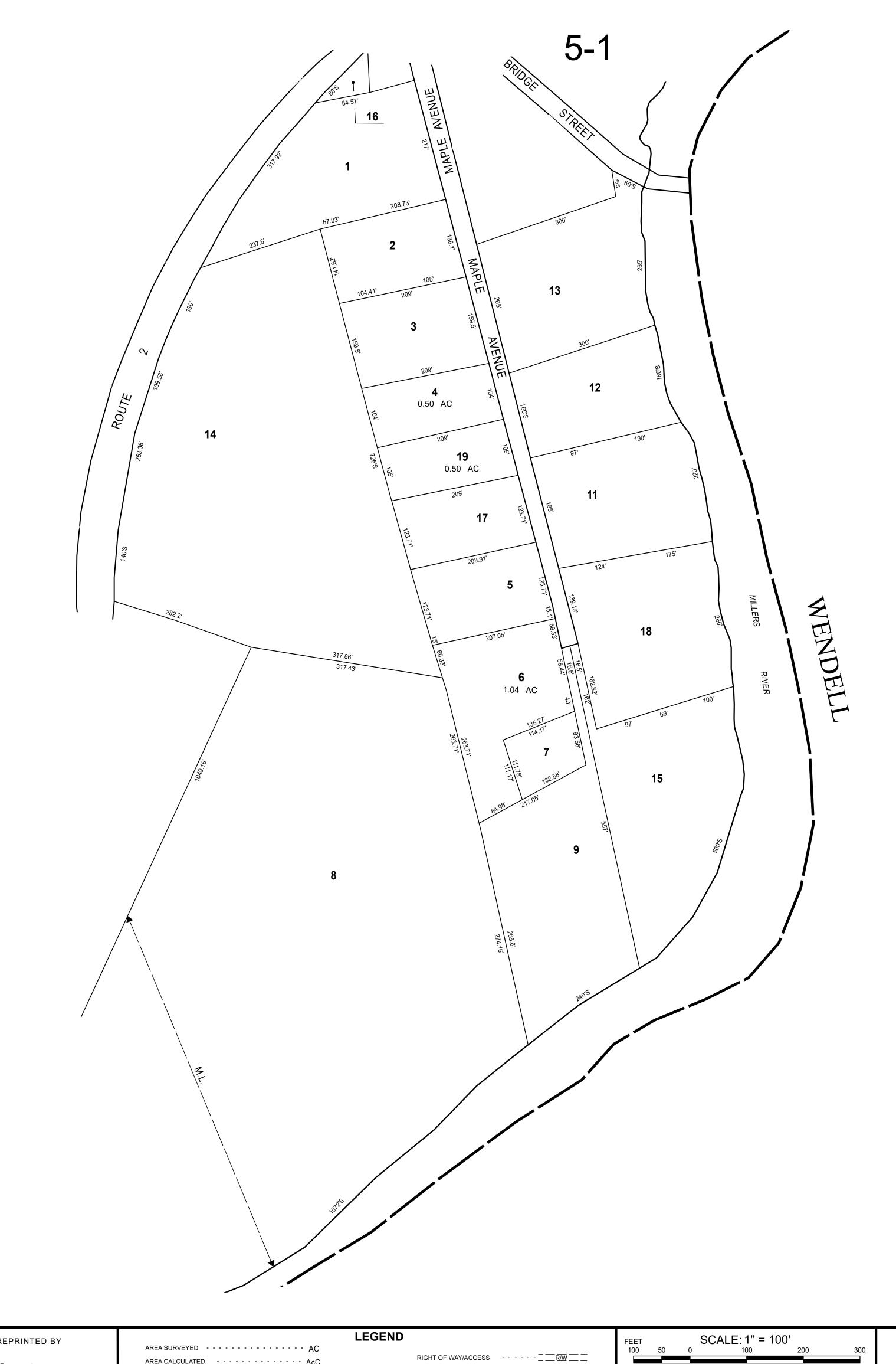
THE HORIZONTAL DATUM IS THE MASSACHUSETTS STATE PLANE COORDINATE SYSTEM, NAD 83.
