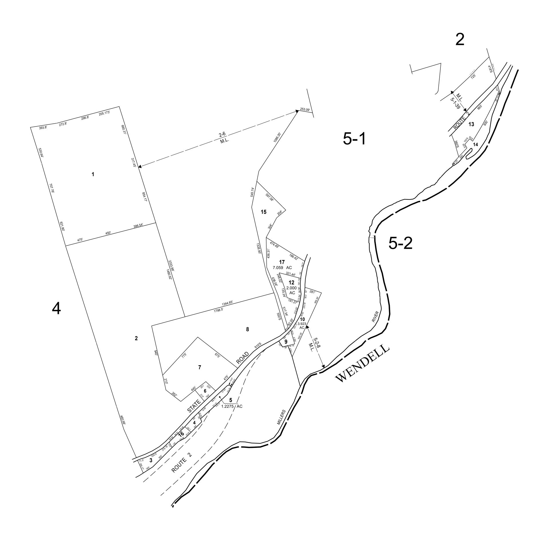
THE HORIZONTAL DATUM IS THE MASSACHUSETTS STATE PLANE COORDINATE SYSTEM, NAD 83.
