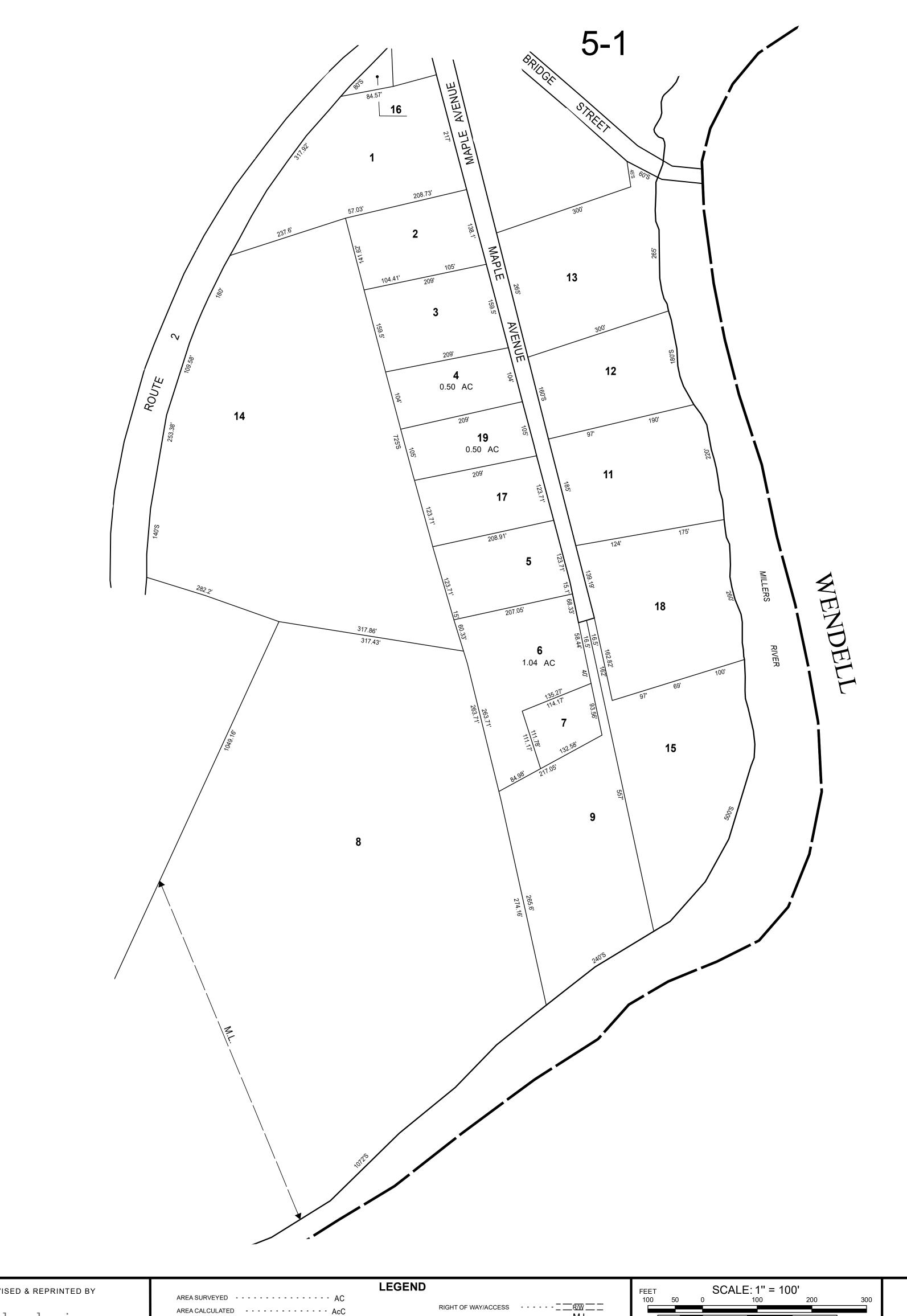
THE HORIZONTAL DATUM IS THE MASSACHUSETTS STATE PLANE COORDINATE SYSTEM, NAD 83.
